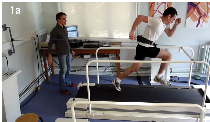
Figure 1: The instrumented sprint treadmill. Subjects are attached to a wall and can accelerate from a still crouched position. It is possible to synchronise electromyography measurements and video motion analysis. 1c) World-class sprinter Christophe Lemaitre sprinting on the treadmill.
